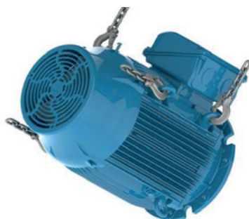
Figure 24 - Motor is being rotated to horizontal position
