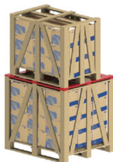
Figure 28 - Use of additional battens for stacking
